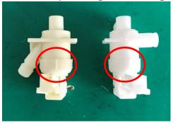
2. Once disassembled from the body, check the rubber boot has no signs of any debris or damage. There is a chance that carbon deposits from the filter can get caught up into the body and cause the rubber boot not to seat correctly onto the housing. The housing itself will also need to be checked for any signs of contaminants or
