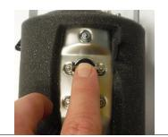
Reattach the metal box by depressing the top flap of the metal box so it snaps back into its original position on the Hot Tank.
